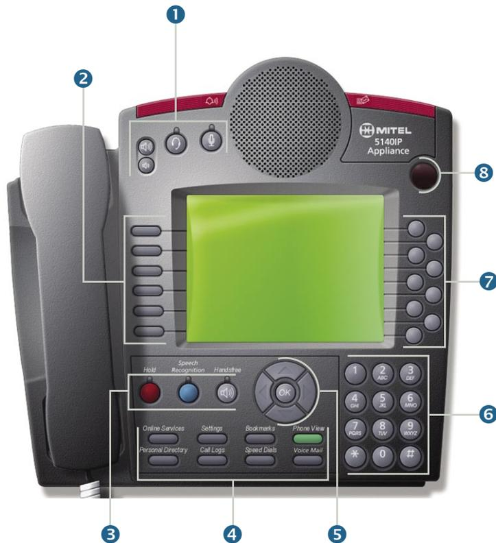
The Mitel Networks™ 5140 IP Appliance provides you with convenient access to powerful features using command keys and quick keys. The Mitel Networks 5140 IP Appliance display screen allows you to easily view and quickly navigate through these features. The full-duplex speakerphone gives you excellent handsfree operation.
